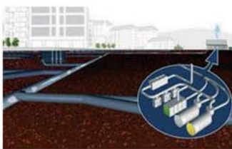
Urban waste collection through an underground vacuum network. Examples exist in Sweden, the Netherlands, Norway, China, and other countries.
