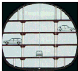
Figure 5. Cross-section of the Landsberg underground car park, Germany: 365 cars or 5,000 people civil defence shelter.
