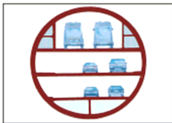
Figure 6. The Bouygues 3-storey MUSE concept: an underground motorway restricted to light vehicles and mass transit in the same 10 m ID tube (designed for the Hauts-de-Seine department, immediately west of Paris, but not yet adopted).
