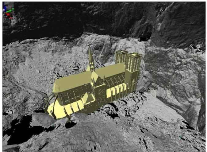
Figure 1: La Verna cave (Pyrénées range) scanned by ATM-3D (volume 3.6 hm<sup>3</sup>)
