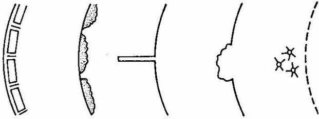
Figure 4: Five tricks to reduce stress concentration around a deep tunnel: centre, deep cut; right, local overbreak or blasted boreholes, left Tauern tunnel shotcrete with uncovered spaces, or wooden planks inserted between concrete blocks
