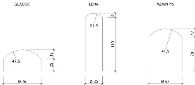
Figure 7: Shapes and dimensions of three axi-symmetrical caverns designed for the LAGUNA experiment (Mosca, 2010)
