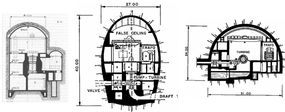
Fig. 1. Three typical cross sections of caverns, at about the same scale: **a**: standard cavern with vertical walls (Lucens nuclear plant, Switzerland, 1966); **b**: ovoid cavern (Porąbka Jar hydro plant, Poland, 1974; **c**: full half circle (Cirata hydro plant, Malaysia, 1980).
