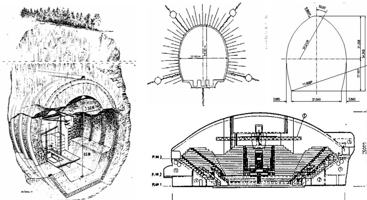
RIB in ROCK: sketch of a construction method for a very large cavern in poor ground Sallström, Sweden, 1977
